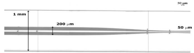
Fig. 5. Photograph of the constricted capillary used as a model of a pore body-pore throat geometry.
